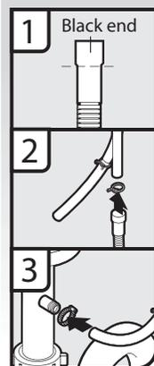
1. Connect black end of drain hose to air gap and cut if needed.
